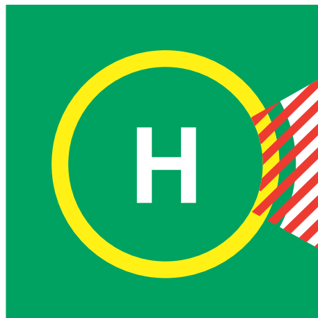
Figure 5-5. Helideck prohibited landing sector marking
